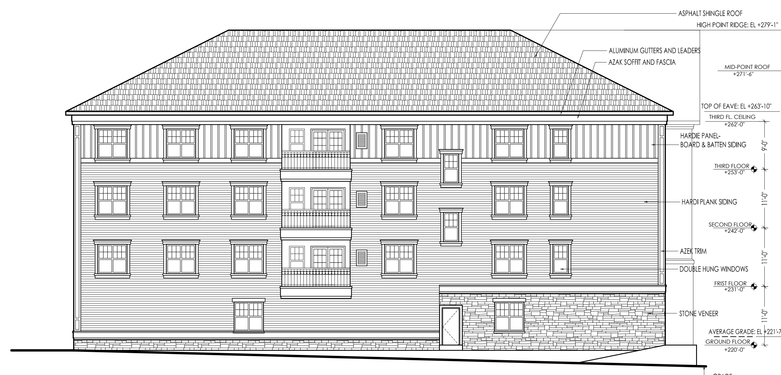
B EAST ELEVATION 3/32" = 1'-0"
